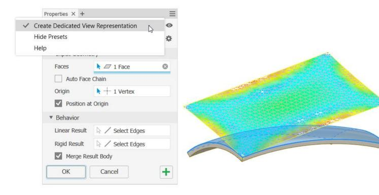
**Tip:** Suppress the embossed features on a sheet metal part to calculate the flat pattern and then unsuppress and selectively unwrap the embossed areas.
